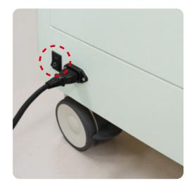
3 Turning on the simulation unit
