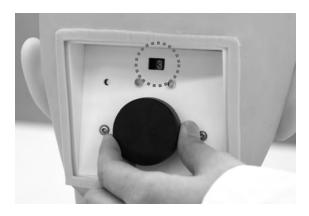
The cases can be switched over by the switch dial. The number appears in the window indicates the chosen case. Refer the table on the quick manual. To practice foreign body removal, set the dial to "FB" and set the "FB Ear" type of external ears. Otherwise, you may damage the ear drum images.
